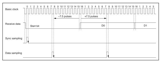
Figure 10.18 Sampling Timing (Asynchronous mode)
