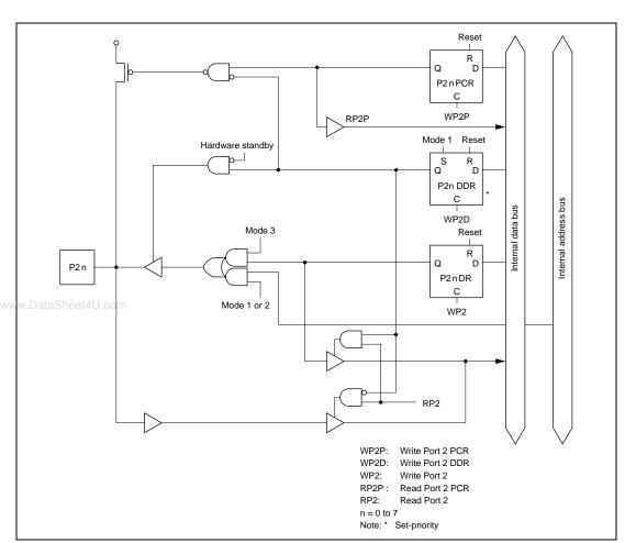
Figure 6.2 shows a schematic diagram of port 2.
