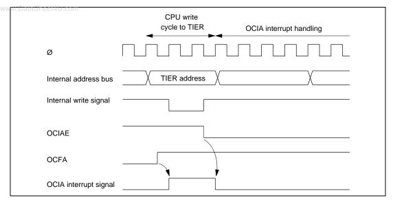
Figure 4.7 shows an example in which the OCIAE bit is cleared to "0."
