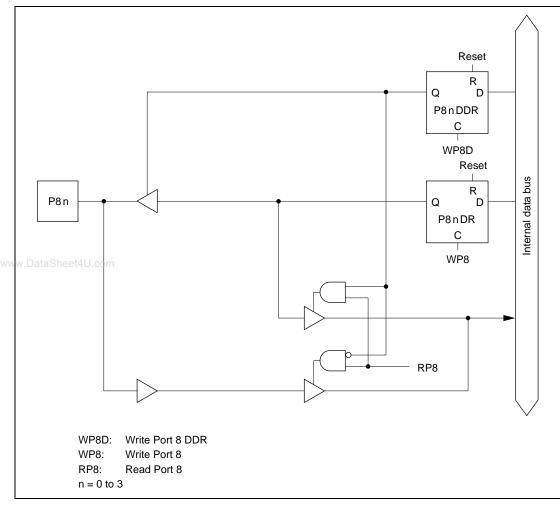
Figure 6.8 (a) Port 8 Schematic Diagram (Pins P8, to P8,)
