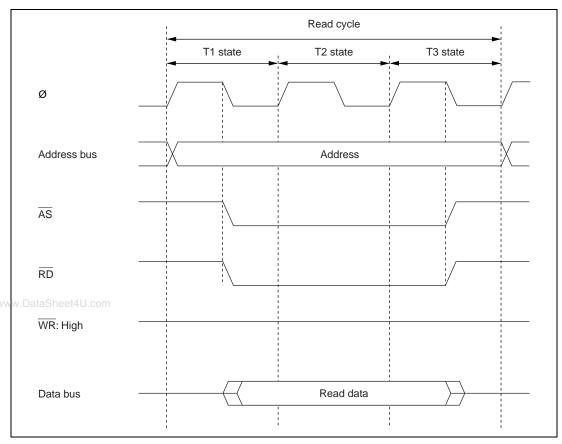
Figure 2.17 (a) External Device Access Timing (Read)
