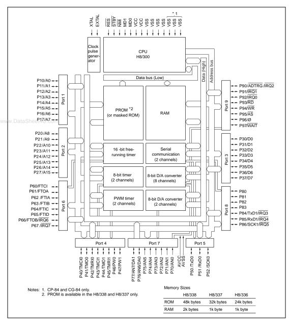
Figure 1.1 Block Diagram
