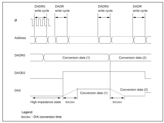
Figure 12.2 D/A Conversion (Example) www.DataSheet4U.com
