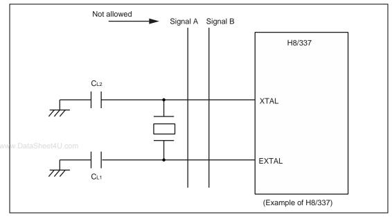
Figure 5.4 Notes on Board Design around External Crystal
