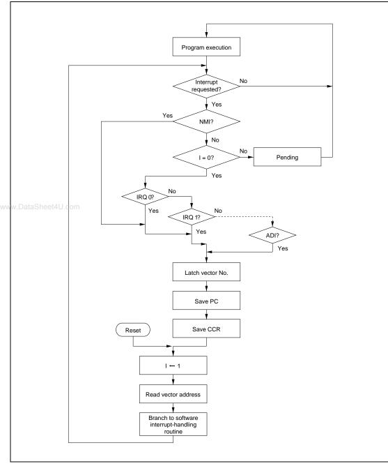
Figure 4.4 Hardware Interrupt-Handling Sequence
