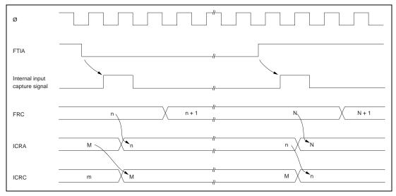
Figure 7.10 Input Capture Timing (Usual case)
