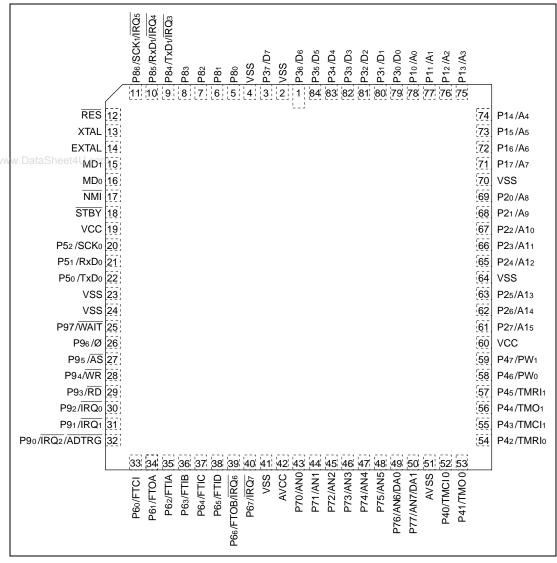
Figure 1.2 Pin Arrangement (CG-84, Top view)
