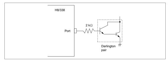
Figure 16.1 Example of Circuit for Driving a Darlington Pair (5V Version)
