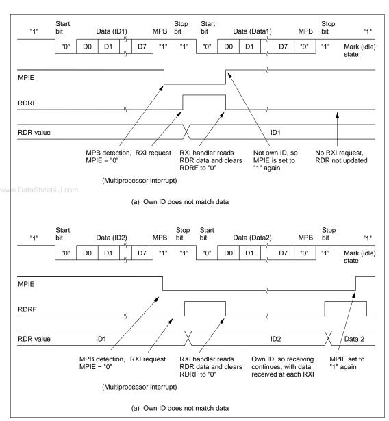
Figure 10.11 shows an example of SCI receive operation using a multiprocessor format.
