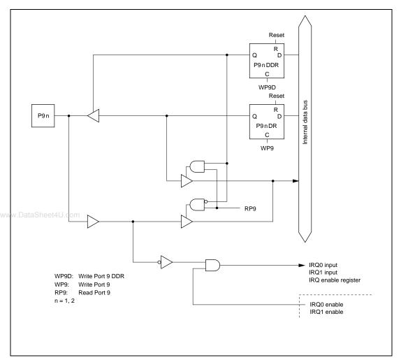
Figure 6.9 (b) Port 9 Schematic Diagram (Pins P9, and P9,)
