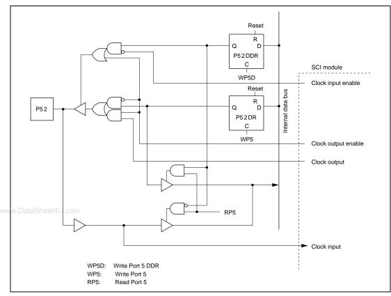
Figure 6.5 (c) Port 5 Schematic Diagram (Pin P5<sub>2</sub>)
