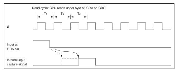
www.DataSheet4U.com Figure 7.11 Input Capture Timing (1-State delay)
