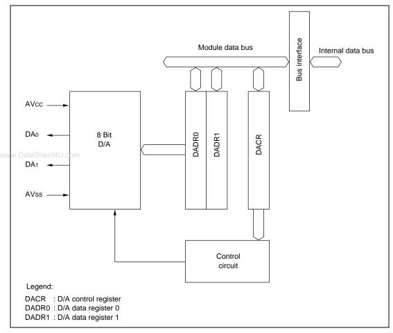
Figure 12.1 D/A Converter Block Diagram
