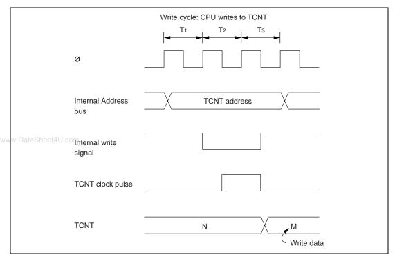
Figure 8.11 TCNT Write-Increment Contention
