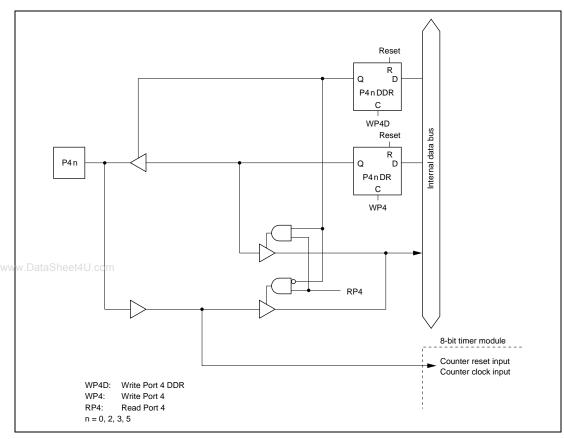
Figure 6.4 (a) Port 4 Schematic Diagram (Pins P4<sub>0</sub>, P4<sub>2</sub>, P4<sub>3</sub>, and P4<sub>5</sub>)
