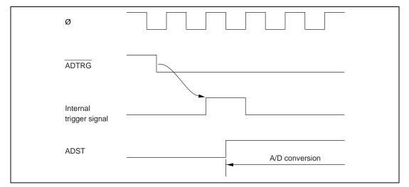
Figure 11.5 External Trigger Input Timing
