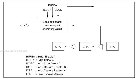
Figure 7.2 Input Capture Buffering
