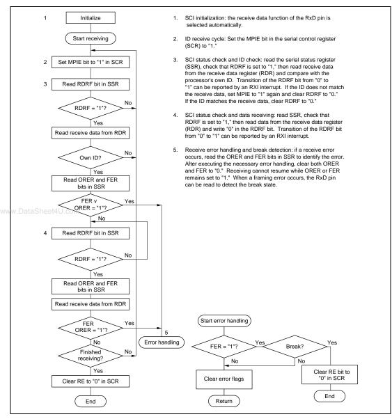
Figure 10.10 Sample Flowchart for Receiving Multiprocessor Serial Data
