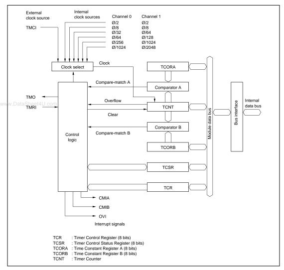
Figure 8.1 Block Diagram of 8-Bit Timer
