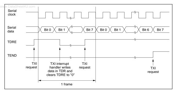
Figure 10.14 shows an example of SCI transmit operation.
