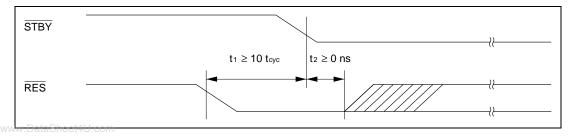
(2) When the RAME bit in SYSCR is set to "1" or when it is not necessary to retain RAM contents, RES does not have to be driven low as in (1).
