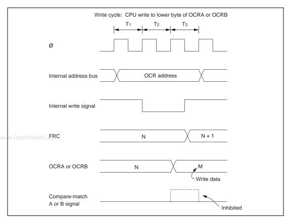
Figure 7.18 FRC Write-Increment Contention
