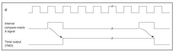
Figure 8.5 Timing of Timer Output
