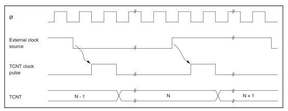
Figure 8.3 Count Timing for External Clock Input
