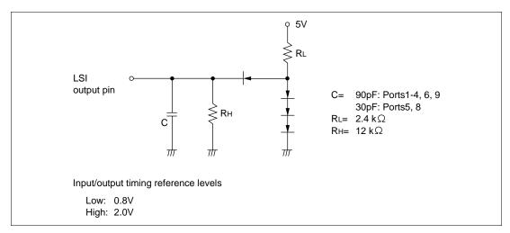
Figure 16.3 Output Load Circuit
