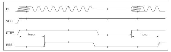
Figure 16.8 Clock Settling Timing
