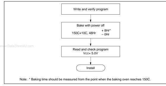
Figure 14.7 shows the recommended screening procedure.
