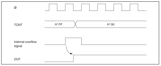
Figure 8.8 Setting of Overflow Flag (OVF)
