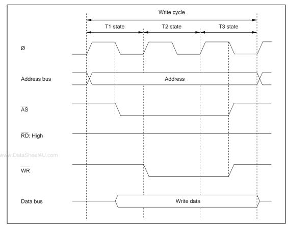
Figure 2.17 (b) External Device Access Timing (Write)
