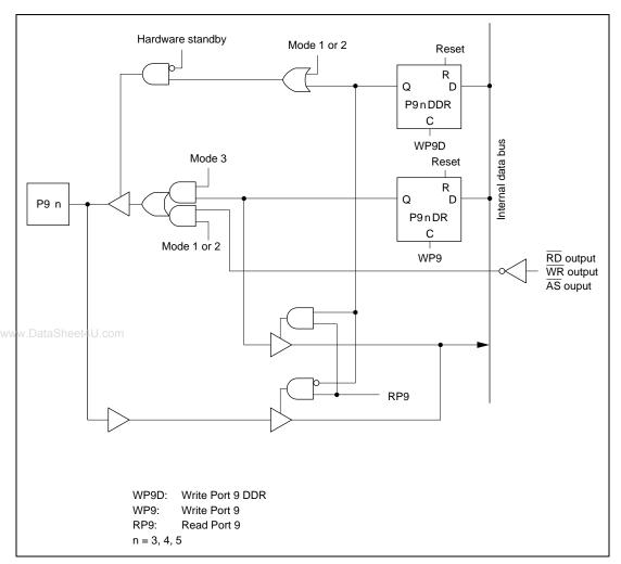
Figure 6.9 (c) Port 9 Schematic Diagram (Pins P9<sub>3</sub>, P9<sub>4</sub>, and P9<sub>5</sub>)
