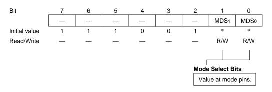
Note: \* Determined by inputs at pins MD1 and MD0
