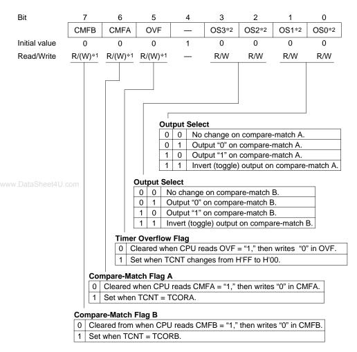
Notes: 1. Software can write a "0" in bits 7 to 5 to clear the flags, but cannot write a "1" in these bits. 2. When all four bits (OS3 to OS0) are cleared to "0," output is disabled.
