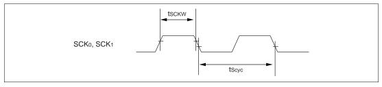
Figure 16.17 SCI Input Clock Timing
