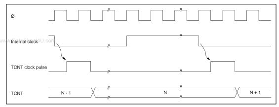
Figure 8.2 Count Timing for Internal Clock Input
