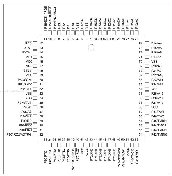
Figure 1.3 Pin Arrangement (CP-84, Top view)
