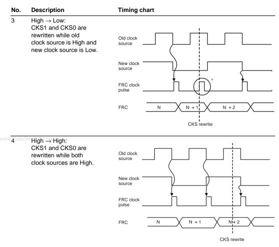
Note: The switching of clock sources is regarded as a falling edge that increments the FRC.
