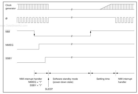
Figure 15.1 NMI Timing in Software Standby Mode
