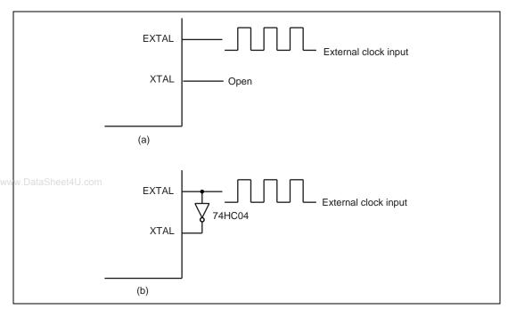
Figure 5.5 External Clock Input (Example)
