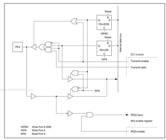
Figure 6.8 (b) Port 8 Schematic Diagram (Pin P8<sub>4</sub>)
