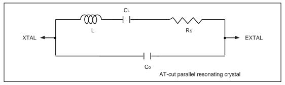
Figure 5.3 Equivalent Circuit of External Crystal
