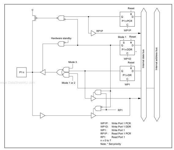
Figure 6.1 Port 1 Schematic Diagram
