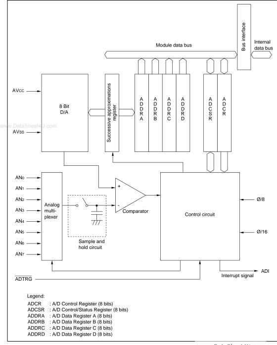
Figure 11.1 Block Diagram of A/D Converterw.DataSheet4U.com
