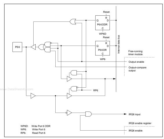
Figure 6.6 (c) Port 6 Schematic Diagram (Pin P6<sub>6</sub>)
