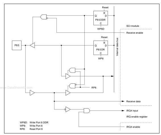
Figure 6.8 (c) Port 8 Schematic Diagram (Pin P8<sub>5</sub>)
