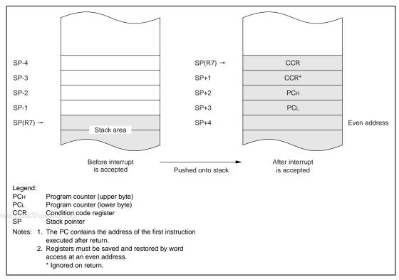
Figure 4.5 Usage of Stack in Interrupt Handling
