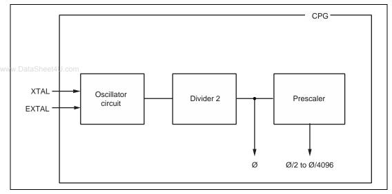
Figure 5.1 Block Diagram of Clock Pulse Generator
