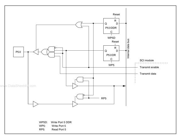
Figures 6.5 (a) to 6.5 (c) show schematic diagrams of port 5.
