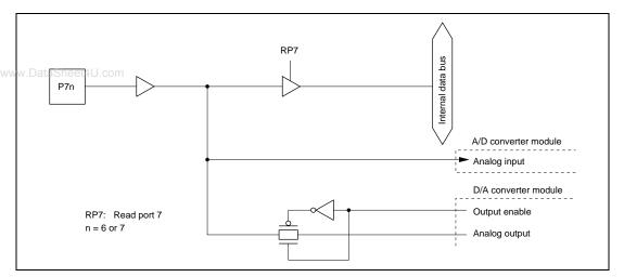
Figure 6.7 (b) Port 7 Schematic Diagram (Pins P7, and P7,)
