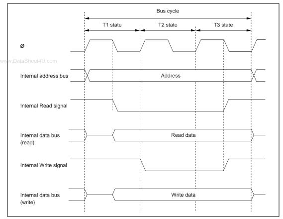
Figure 2.15 On-Chip Register Field Access Cycle
