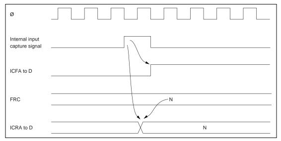
Figure 7.12 Input Capture Timing (1-State delay, buffer mode)
