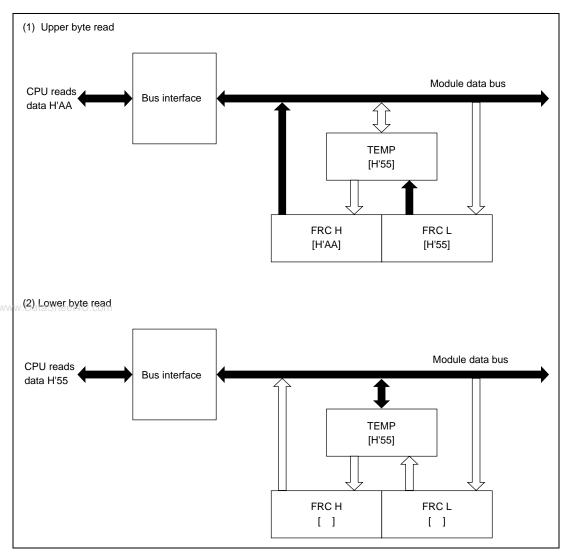
Figure 7.3 (b) Read Access to FRC (when FRC contains H'AA55)
