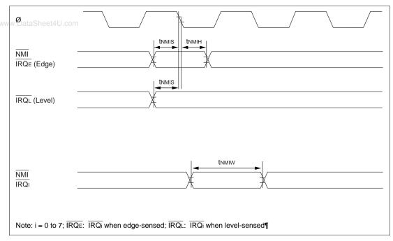
Figure 16.7 Interrupt Input Timing
