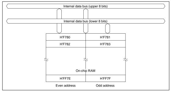
Figure 13.1 Block Diagram of On-Chip RAM (H8/338)
