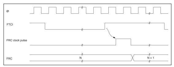
Figure 7.5 Increment Timing for External Clock Source
