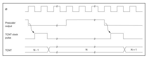
Figure 9.2 TCNT Increment Timing
