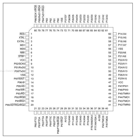
Figure 1.4 Pin Arrangement (FP-80A, Top view)
