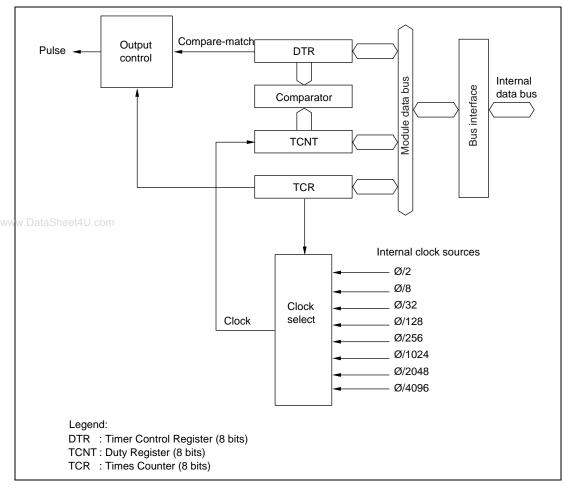
Figure 9.1 Block Diagram of PWM Timer
