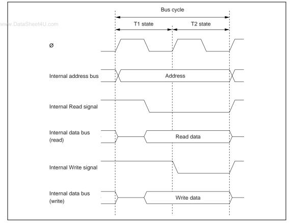
Figure 2.13 On-Chip Memory Access Cycle
