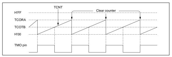
Figure 8.9 Example of Pulse Output
