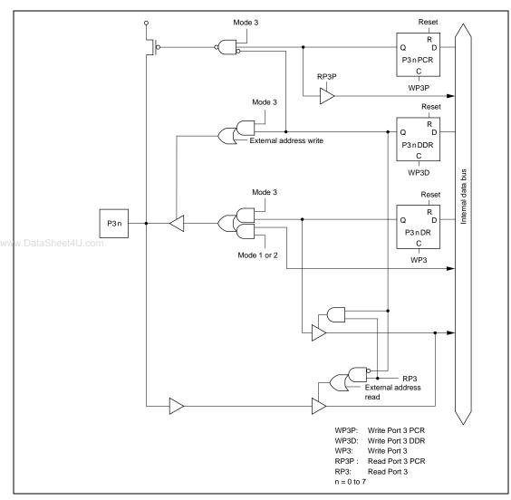
Figure 6.3 Port 3 Schematic Diagram
