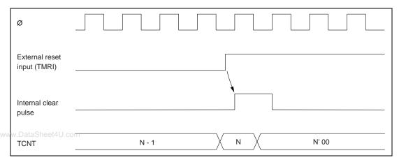
Figure 8.7 Timing of External Reset
