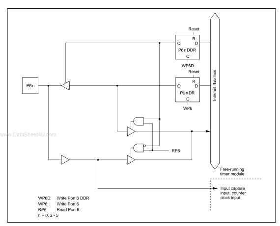
Figure 6.6 (a) Port 6 Schematic Diagram (Pins P6, P6, P6, P6, P6, and P6,
