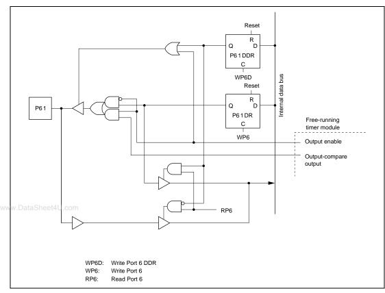
Figure 6.6 (b) Port 6 Schematic Diagram (Pin P6<sub>1</sub>)
