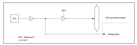
Figure 6.7 (a) Port 7 Schematic Diagram (Pins P7, to P7, t
