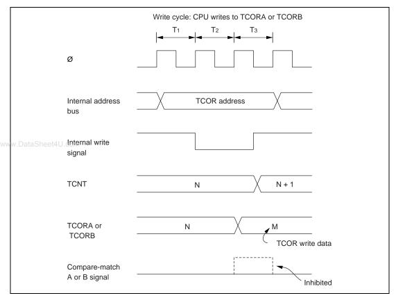
Figure 8.12 Contention between TCOR Write and Compare-Match
