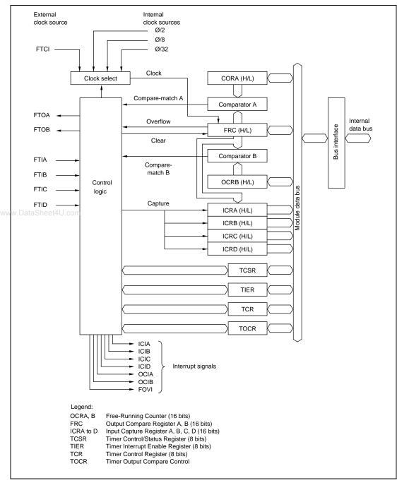
Figure 7.1 Block Diagram of 16-Bit Free-Running Timer
