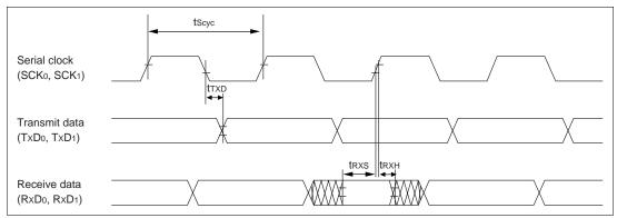
Figure 16.16 SCI Input/Output Timing (Synchronous mode)
