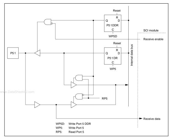
Figure 6.5 (b) Port 5 Schematic Diagram (Pin P5<sub>1</sub>)
