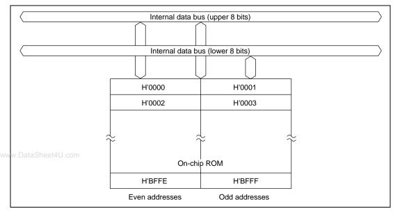
Figure 14.1 is a block diagram of the on-chip ROM.
