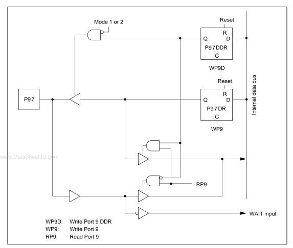
Figure 6.9 (e) Port 9 Schematic Diagram (Pin P9<sub>7</sub>)
