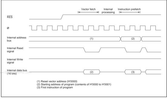
Figure 4.1 Reset Sequence (Mode 2 or 3, Program Stored in on-chip ROM)
