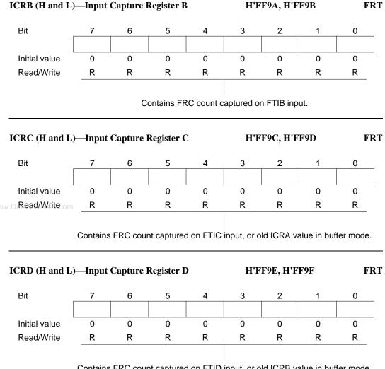
Contains FRC count captured on FTID input, or old ICRB value in buffer mode.
