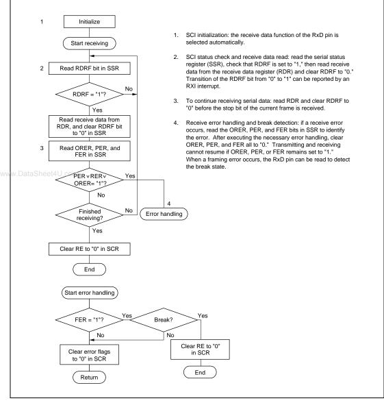
Figure 10.7 Sample Flowchart for Receiving Serial Data
