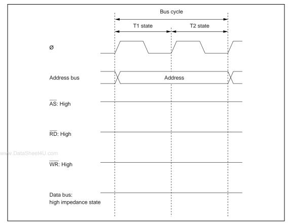
Figure 2.14 Pin States during On-Chip Memory Access Cycle
