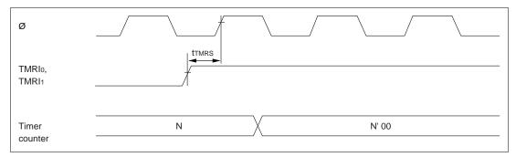
Figure 16.14 8-Bit Timer Reset Input Timing
