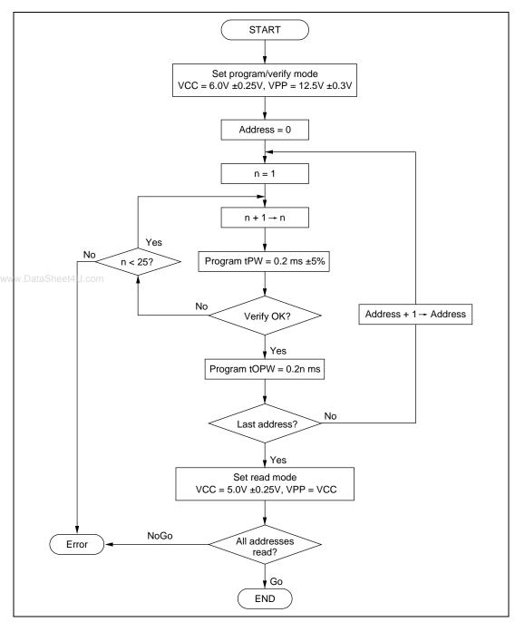
Figure 14.5 High-Speed Programming Flowchart
