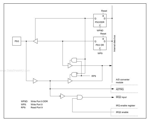
Figure 6.9 (a) Port 9 Schematic Diagram (Pin P9<sub>0</sub>)
