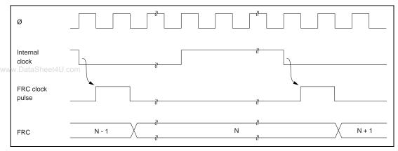
Figure 7.4 Increment Timing for Internal Clock Source
